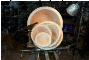
He will be giving a demonstration on hollowing bowls from half logs using Kel McNaughton's Center Saver tools. Being able to cut multiple bowls from a single wood blank offers numerous advantages including increased profitability, lower cost per bowl and is an environmentally sound approach to woodturning.
